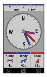
You can use the dog tracking compass to view the direction and distance to your dog, your vehicle, and any paired devices. The dog tracking compass also shows the dog's status, such as running or on point (*Dog Status lcons*, page 13). The color of the pointer corresponds to the color of the track.
